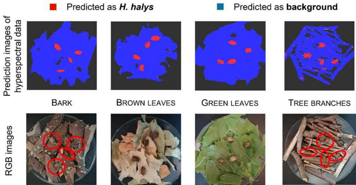
In the frame of **HALY.ID** project, the present study aims at investigating the potential of near-infrared spectral cameras for monitoring the presence of the brown marmorated stink bug (*Halyomorpha halys*) in crop fields.
