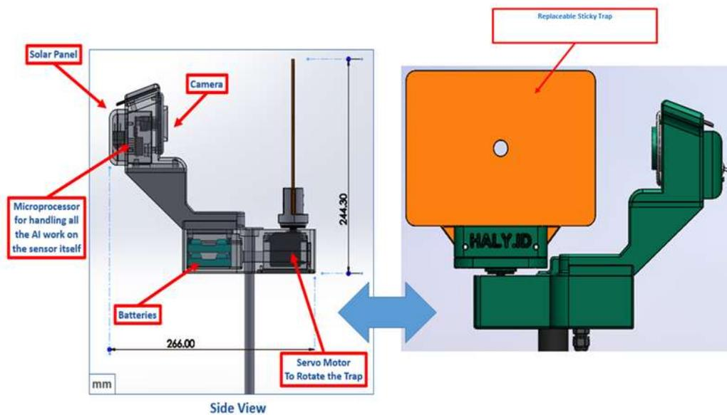
*Halyomorpha halys* (HH), is an invasive shield native to East Asia. Due to climate change and global trade, it has arrived in Europe where it is causing significant losses in food production. As part of the HALY.ID project, we propose to develop a novel smart trap for automated insect monitoring.
