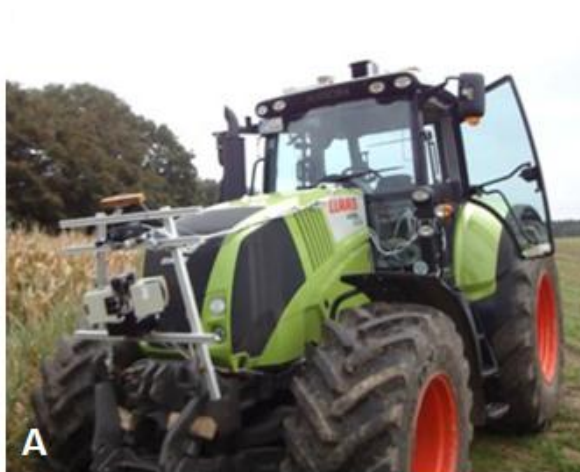
Ambient Awareness for Autonomous Agricultural Vehicles (QUAD-AV): Tractor with RADAR and odometer, rotating LIDARs, stereo cameras and thermographic camera (A); and view from a thermographic camera, in which a person hiding in a maize field is clearly visible (B). ICT-AGRI Project.
